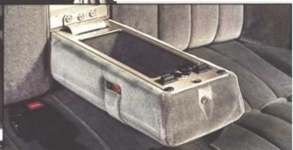
The foldable armrest houses controls for the reading lamps and the volume control for the stereo loudspeakers. Space is provided for a telephone.
