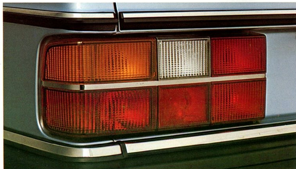
Distinctive 264 rear light assembly includes rear fog lights.
