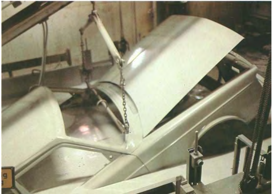
First stage of the extensive body treatment, electrolytic primer bath.
