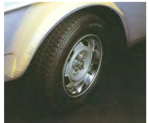
Polypropylene inner liners for front wheel housings protect against dirt and moisture as well as flying stones and gravel.
