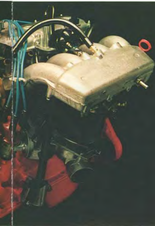
THE B21 F IS A 2.1 LITER IN-LINE FOUR WITH AN OVERHEAD CAM AND FUEL INJECTION.
