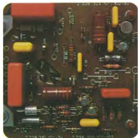
SOLID STATE IGNITION PROVIDES A HIGH QUALITY IGNITION PULSE AND EXACT TIMING FOR EFFICIENT COMBUSTION.
