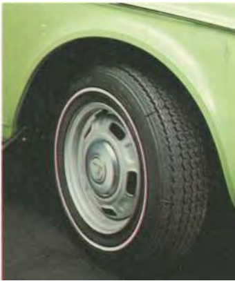
(Left) Steel-belted radial tires have less rolling resistance for longer tread life and greater gas mileage.
