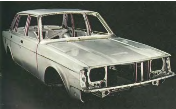
(Left) Fully-welded Volvo safety body combines box profiles to form a protective cage around the passengers.
